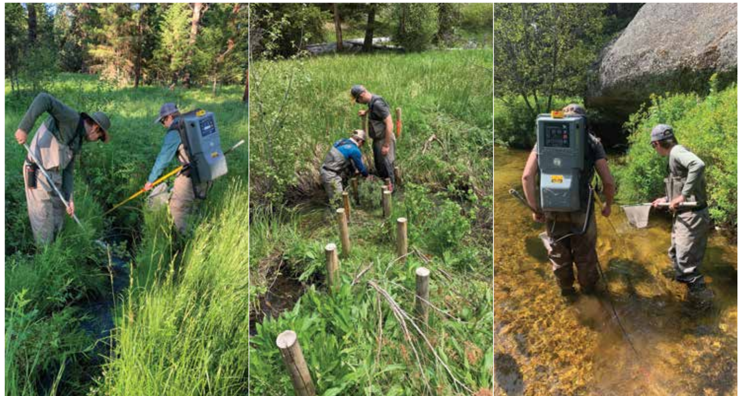
Right: Scientists use backpack electrofishing units and inspections to measure the impact of BDAs on fisheries and water flows.
